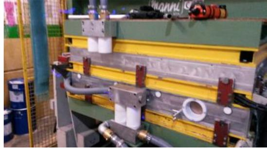
Each side mold will be equipped with connections for connecting the cavity to the vacuum plant, vacuum distribution in the whole cavity and a dedicated injection holes able to maintain the vacuum level even at the insertion of the injection head.
