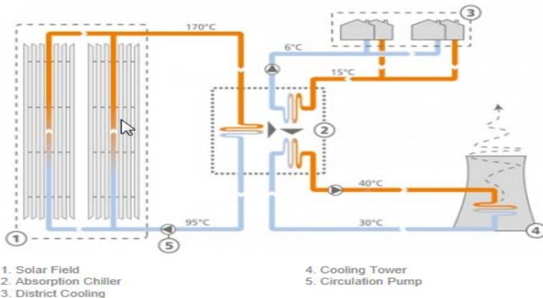
The increasing requirement for cooling can be produced most economically by district cooling systems with a correspondingly large solar field. The cooling energy is carried to the respective consumers in transmission line networks. District cooling systems are becoming the popular choice in high temperature locations including the Middle East. Novatec Solar's system provides the sustainable solution to the district cooling and refrigeration demands of these regions.
