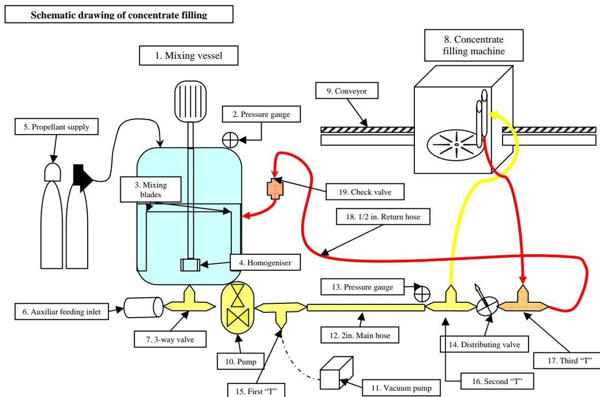
Note: Numbers are referred to "Schematic drawing of concentrate filling machine" drawing below.
