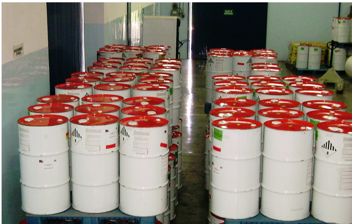
Figure 5 Unwanted ODS stockpiles from pharmaceutical industries generated after phase-out of CFC blends used as propellants in meter-dosed inhalers
