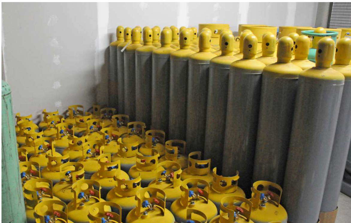
Figure 9 Unwanted CFC-12 recovered
