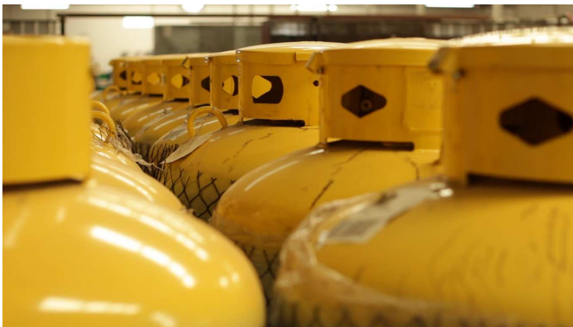
Figure 12 Aggregation containers for ODS consolidation, storage and handling
